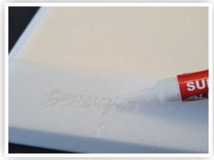
Apply supa glue to the beveled edge about 50mm down from the top corner on both sides
