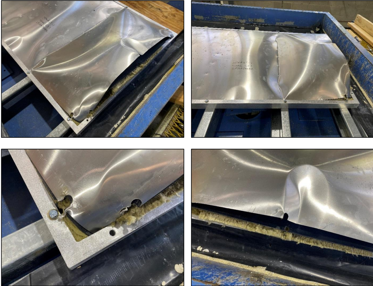
Figure 5: Typical damage after Trial SS1
